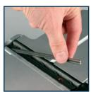
2. Remove the planer blade (9) from the slot in the blade barrel (10) in which it is retained.
